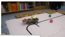
Moving Robot picking up color balls Using H8S/2377 MCU (Final Year Student project)
