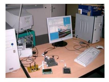
Up to 200 hours practical work per year in Polytech Clermont-Ferrand Lab based on M32C + real-time kernel to drive a specific simulation car game on PC
